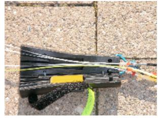
Open the LineCrawler and place each line in a channel.
