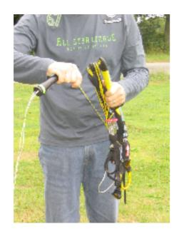
As you wind the lines you can hold the LineCrawler to help you keep the lines winding and assist the untangling of the lines.
