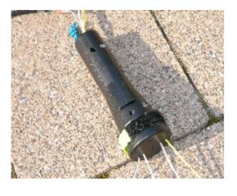
Now close the LineCrawler and fasten the velcro strap around the front of the LineCrawler to secure both halves together.
